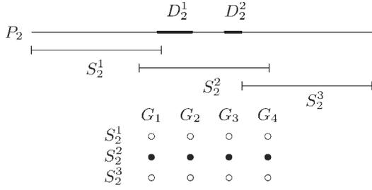
**Fig. 3.** A scenario where the Multiple-Profile method fails to identify domain-level co-evolution. Since the two separate domains  $D_2^1$  and  $D_2^2$  are covered together by segment  $S_2^2$ , their individual phylogenetic profiles do not appear in the segment phylogenetic profiles. As no a priori information is available on the size and location of the domains, it is not possible to avoid such situations using fixed-size segments.
